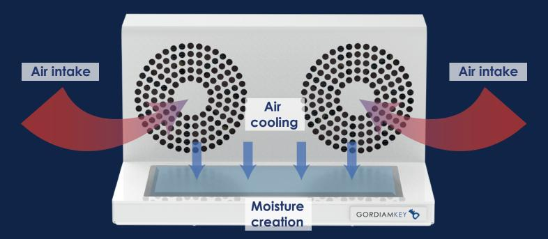
Air at room temperature is constantly transported into the coldplate by the fans.
